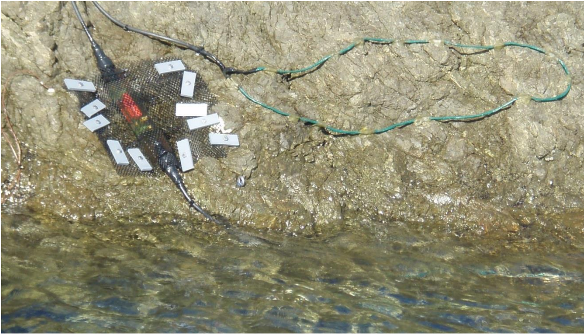
Figure B.1 Photo of antenna components mounted to rocky intertidal shoreline
